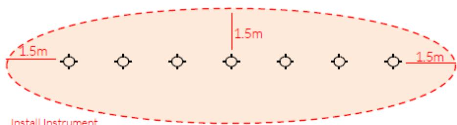
Install Instrument with 1.5m free space (from widest point) around it.
