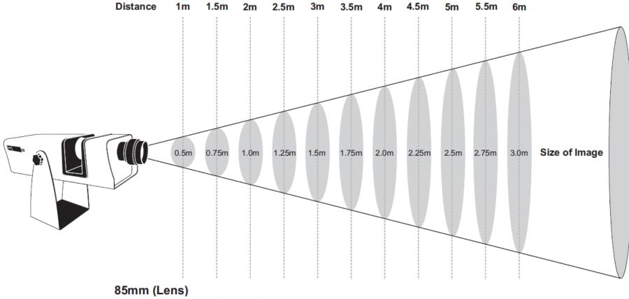
Ratio for Distance 2:1 (Image Size - 85mm Lens) The Object Diameter is 42mm
