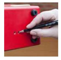
Don't press too hard; you should feel a gentle click like on a keyboard or doorbell. Only after holding the control for <u>5 seconds</u> the volume will begin to increase or decrease, so it can be set to the appropriate level.
