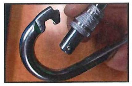
The locking nut of the Safety Snap should not move from side to side at any great angle. If it does, discontinue use immediately.
