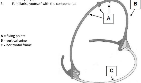
The frame consists of 5 main tubular parts, 6 adjustable feet and a fixing set.
