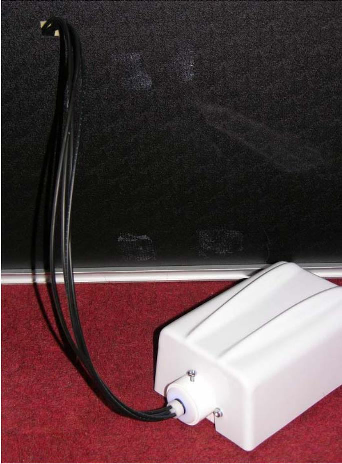
2. Connect the power lead into the back of the Light Source. Plug in at the wall and switch on. Once you have seen the lights come on, unplug. The lights will only be visible on one side. The side with the lights should face the floor; the smooth side with the wires and boss coming out of it is the back and should face the ceiling.
